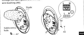
· Secure the luminaire to the wall with the M4.5 screw (A1), rubber ring (A8) and the screw raw plug (A2). The screws and cover should be installed properly to ensure the waterproof protection.
