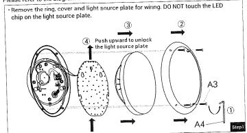
Put the light source plate back on one of the studs to ensure the light source plate will not dangling freely and prevent wire damage during installation.
